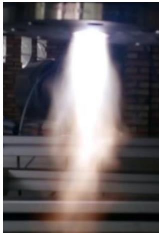
5 6 Fig. 1. Plasma flame as a downflow free jet in open 7 atmosphere at 50 L/min air with P=3600 W
